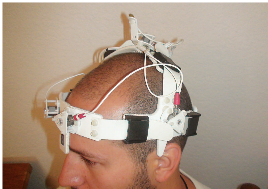
A prototype device developed by retired U.S. Navy sonar experts, using submarine technology, could become a new paradigm for the detection, diagnosis and monitoring of stroke. Above: a headset and laptop-based console can be used to detect, identify and locate a stroke or brain trauma with high sensitivity and specificity without radiation.
